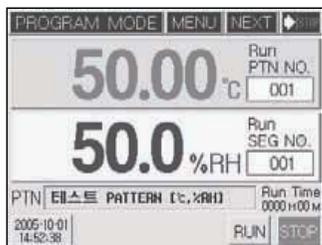
(Fig.20) The 1st running screen of program control(Stop screen)
