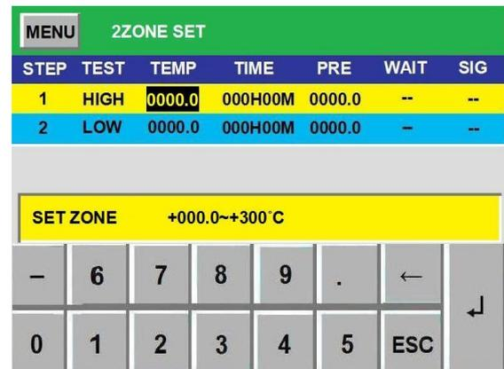
Setting step 1 : set temperature SV of testing, please confirm the range of SV and input value by on-screen keyboard
