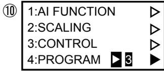
Change menu No. into 4 with the **DIAL**, and press the **ENT**. It moves to the quantity of patterns display.
