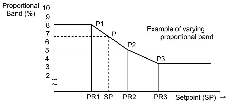
An output limit is the same as that of PID. However, unlike PID, the computation mode in case SP is RP1 or less or RP3 or more, it varies on the same straight line between RP1-RP2 and as between RP2-RP3, respectively. The polygonal line of an upper limit and a lower limit of operation becomes as it is shown in the following figure.
