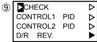
Check and change the control mode (CONTROL), and control direct /reverse action (D/R). A changing procedure is the same as ①. In case of dual output (option) nothing, CONTROL2 is not displayed. Moreover, in case of dual output, changing the control direct/reverse action cannot be performed. If the **ENT** is pressed several times as CHECK, it will return to a setup menu screen.
