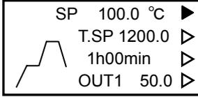
This screen displays 5 steps including current steps. You can confirm execution steps all the time on this display. Scrolls up and down, left and right automatically everytime steps switch.
