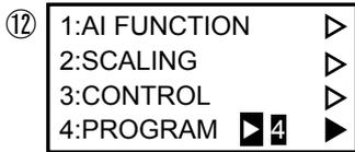
Checking and changing of a basic function are completion above. By changing menu No., check and change other functions, or it returns to an Operation screen by pressing the **DISP**.
