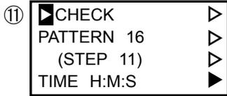
Check and change the quantity of patterns (PATTERN) and a time unit (TIME). A changing procedure is the same as ①. If the **ENT** is pressed several times as CHECK, it will return to a setup menu screen.
