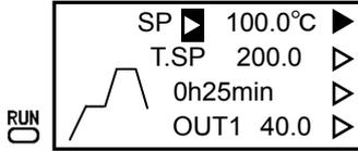
The program stops and the RUN Lamp lights out. At this moment, the SP value is held at the value just before STOP and residual time stops decreasing.
