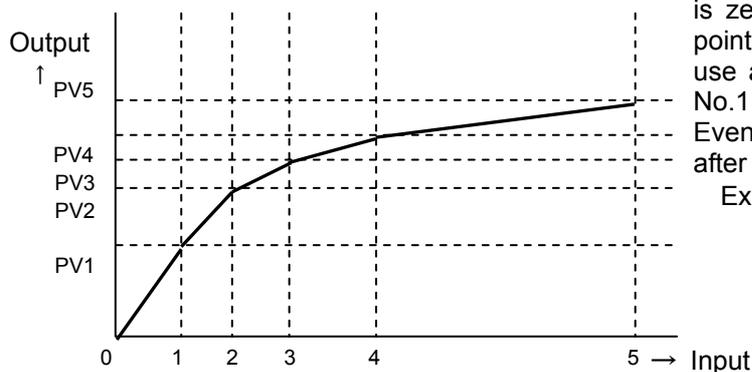
If setting input at the polygonal line point is zero except No.0, that polygonal line point is invalid. Polygonal line points for use are No.0 (always for use) and after No.1 until invalid polygonal line point. Even if setting input is zero, it is invalid after that.
