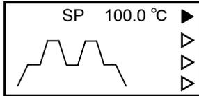
This screen displays 15 steps including current steps. This display scrolls up and down, left and right automatically as done by the partial display. It is shown on Operation (sub) screen at the time of factory settings.
