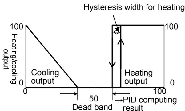
3) PID for 1st output, ON-OFF control for 2nd output
